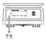
Only weighing platforms that have been levelled precisely horizontally provide accurate weighing results. Weights and Measures approved weighing platforms have a spirit level to simplify levelling.
